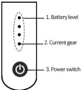
1. Battery indicator: There are four lights to indicate the battery level. Every light represent about 25% power.
