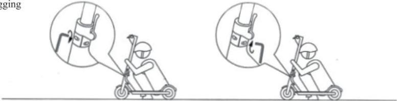
If the pipe shakes, use the Allen wrench to fasten the two screws on the folding mechanism.
