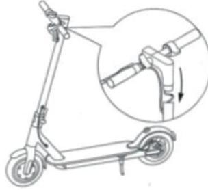
3. Use the Allen wrench to tighten the screws on both sides.
