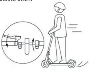
4. Release the accelerator to slow down, energy recovery system will be automatically activated. Squeeze the brake lever at the left handle bar to stop the scooter.
