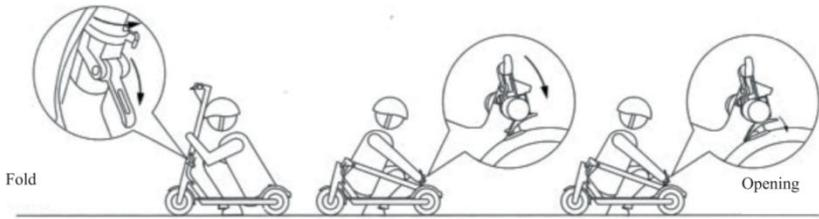
Make sure that the power of electric scooter is turned off, open the folding mechanism, put down the pipe, and hook the handlebars onto the rear fender. When opening you need to press the hook at the rear fender, until the handlebars can be released, then unfold the electric scooter.
