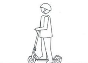
2. Stand on the board with one foot, while the other foot pushes against the ground. After the speed reaches 5km/h, the motor is ready for acceleration.
