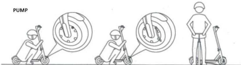
If the tire has gone down, remove the cap on the inlet, connect it to an air pump to inflate it.
