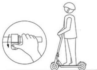
3. Press the accelerator lever slightly, and the scooter accelerates. Put both feet on the board after you can keep balance. Press down the lever to speed the scooter up.
